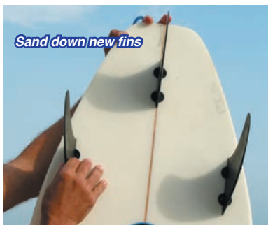
Figure 6.5 Sand down sharp fin edges before use.
