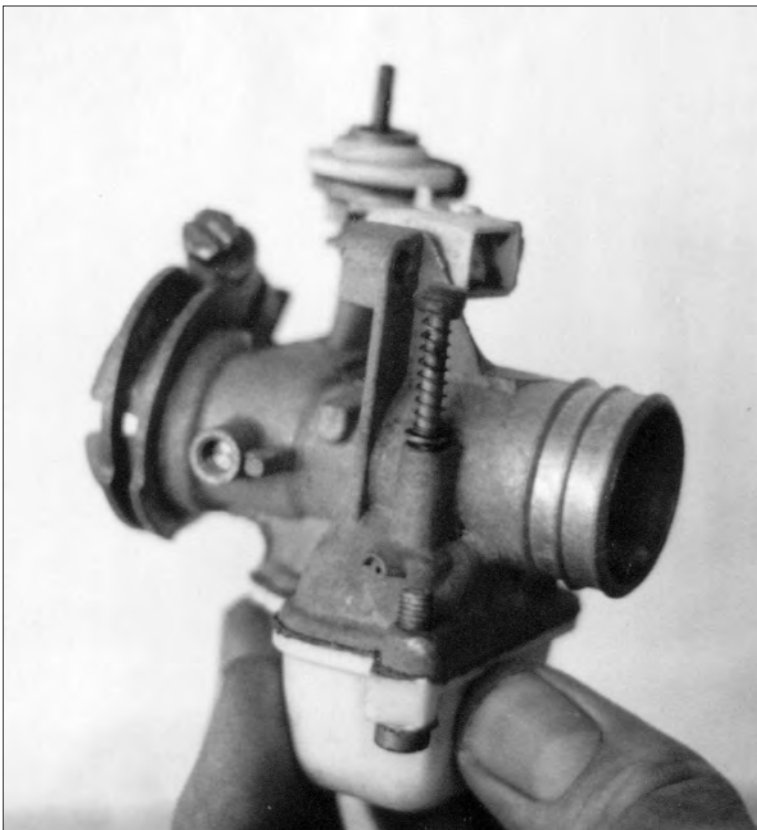
Fig 17 Parts of the carburettor (1) Extension tube (nozzle) (2) Throttle butterfly (3) Venturi (4) Choke Butterfly
