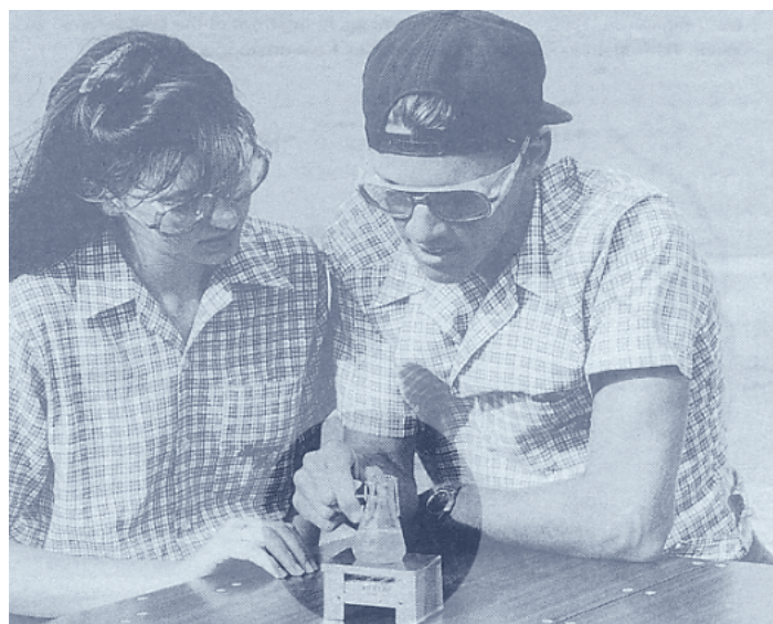
Fig 46 The test involves the use of a hexamine burner kit. If the test is done in a lab, this may be replaced by a bunsen burner
