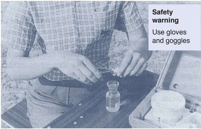
Fig 28 The kit contains chemicals in plastic pillboxes. Use the callipers to cut the top carefully so as not to spill any reagent or get it on your hands or in your eyes
