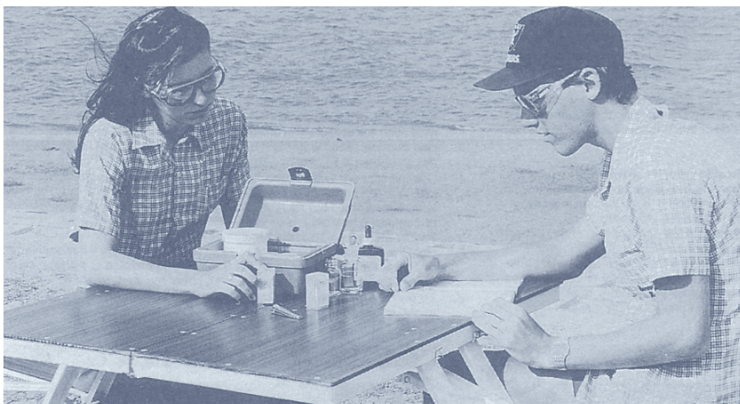
Fig 45 Before you do the Phosphorus test, sit down and read the procedures carefully. It takes about 40-50 minutes to complete and is the longest of the nine tests
