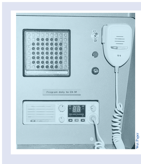
Figure 14.3 A microphone is used to switch between transmit and receive modes
