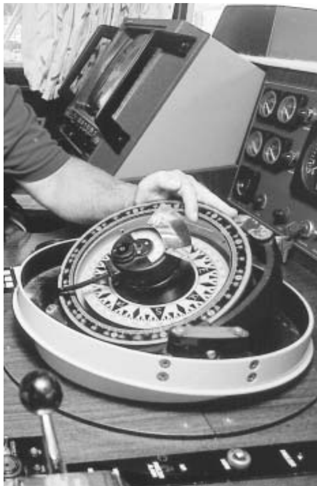
Figure 1.1 Binnacle mounted compass. Note — A binnacle is the pedestal in which a compass is mounted.
