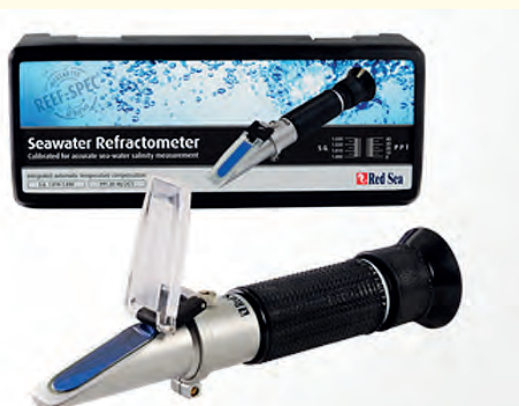
Figure 134.2 A refractometer can also be used to measure salinity Photo Red Sea
